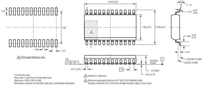
Exact case and lead configuration at supplier discretion within limits shown
